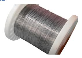
It can not be used in sulphurous and vacuum atmospheres directly at a high temperature, as this will have a significant impact on the EMF values. The composition of positive(KP) is Ni90Cr10, negative(KN) is Ni97Si3.
